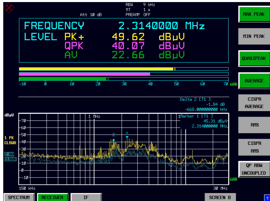
Fig. 4-24 Typical split-screen display
