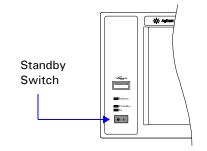
Pressing this front panel switch toggles power to the signal generator between on (green LED on) and standby (orange LED on). In standby mode, the signal generator is switched off, but the instrument is still connected to the line power. The rear panel line switch and the detachable power cord is the instrument disconnecting device. The front panel power switch, therefore, is not, and should not be used as a power switch.
