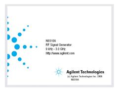
Self-initialization takes about 30 seconds, including self-test. If it detects an error, it reports an error message. The signal generator then defaults to a maximum frequency of 3 GHz and a minimum amplitude of -127 dBm, then the signal generator is ready for your current use. After power on, let the signal generator warm up for 45 minutes for stabilization.
