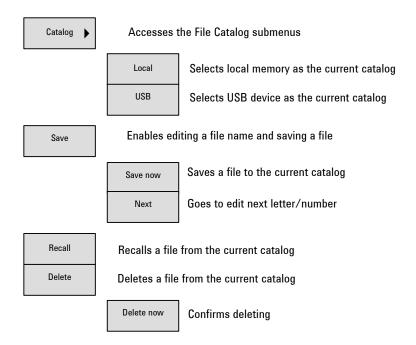
**Catalog** Pressing this softkey selects the catalog for storing configuration files. **Local** means saving a configuration file in the instrument's internal memory. **USB** means saving a configuration file in a peripheral USB memory stick via the USB device connector.
