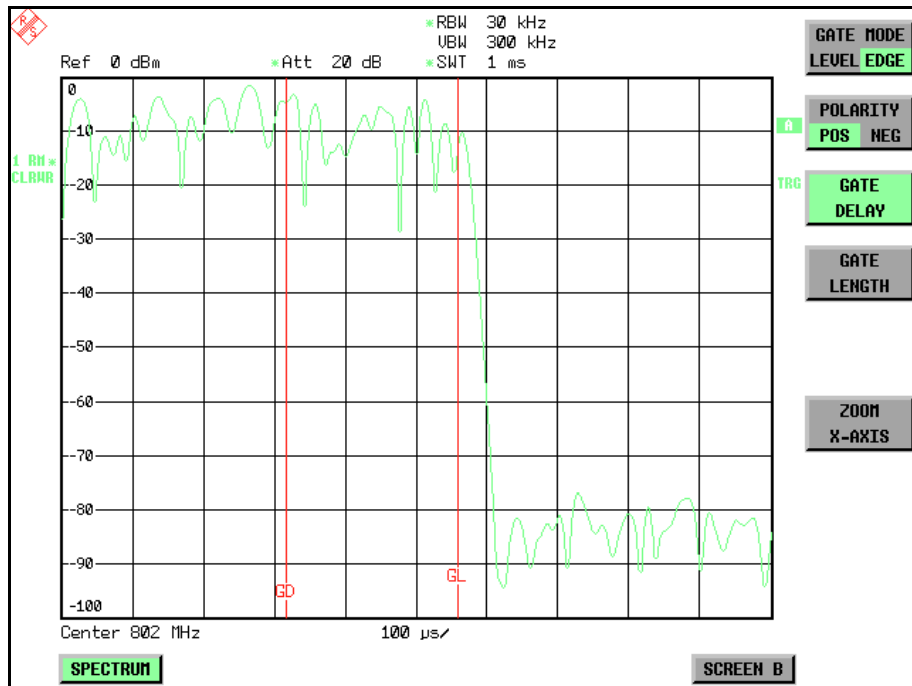
Fig. 4-4 Setting GATE DELAY and GATE LENGTH in time domain by means of lines GD and GL
