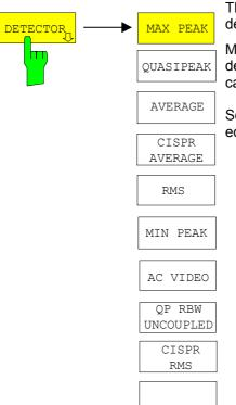
The DETECTOR softkey opens a submenu to select the detector
